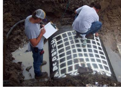
One element of the Board's post Katrina recovery is a Sewer Force Main Reliability Study, a field inspection using ultrasonic testing to determine the pipe wall thickness. The results are compared to the original design thickness of the pipe to determine the condition and remaining service life of the sewer force main. As many as 640 thickness measurements within a predetermined area are taken to complete the process.
